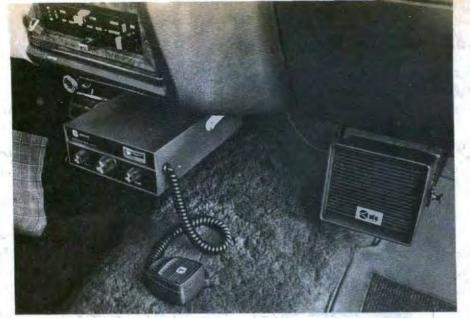
Photo shows external speaker in typical under-dash position.
